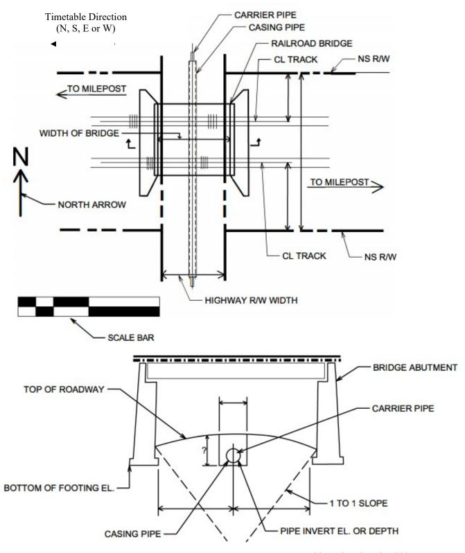
Plate VI - Sample Pipe Plan and Section Under Railway Bridge
