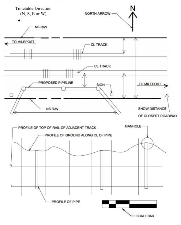
Plate IV - Sample Pipe Parallel Plan and Profile Views
