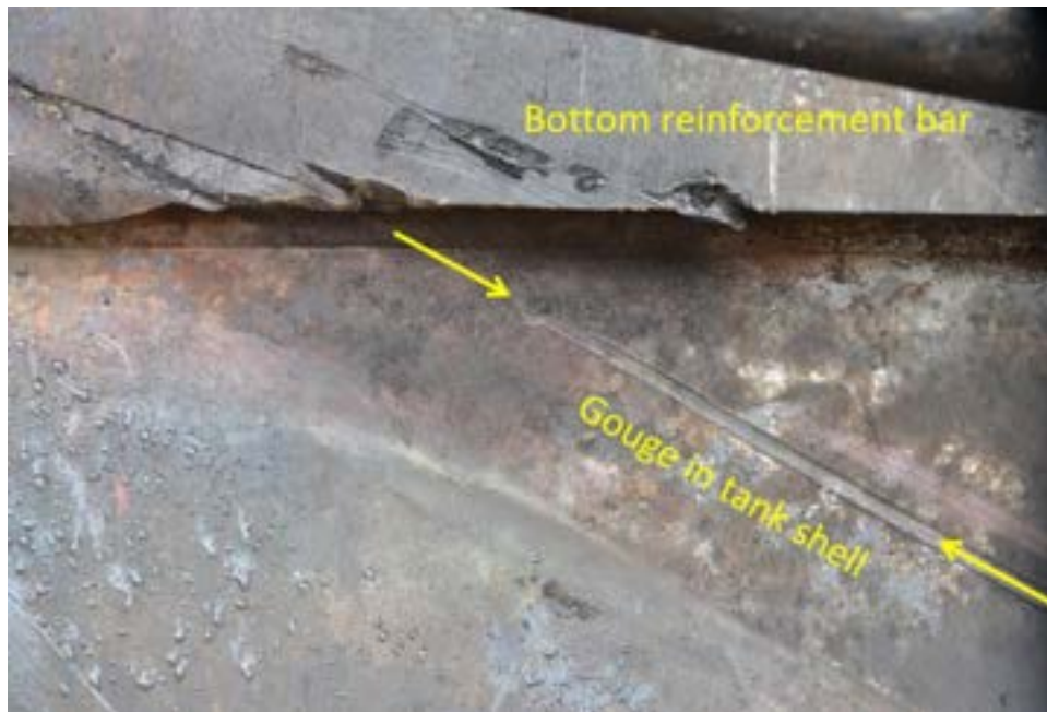
Figure 5 Gouge – indicating removal of metal and a reduction in thickness. 7
