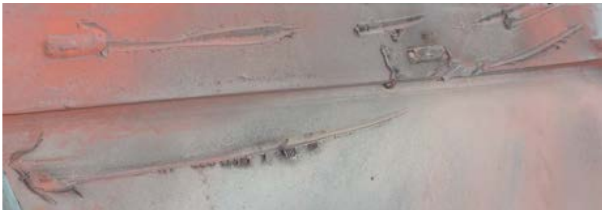
Gouge in bottom reinforcement pad and tank [Casselton, ND 2013].
