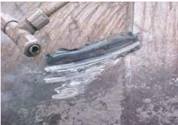
Figure 25 Wheel burn in tank shell. 27
