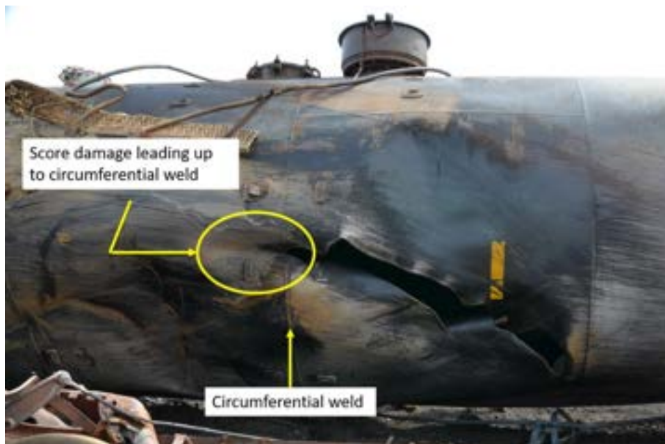
Figure 7 The bolster of an adjacent tank car scored the side of this tank; the body bolster engaged the circumferential weld long enough that the adjacent tank shell stretched, thinned, and initiated the tear that can be observe in the tank. 9
