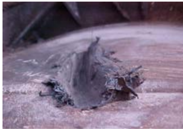
Figure 25 Wheel burn in tank shell. 27
