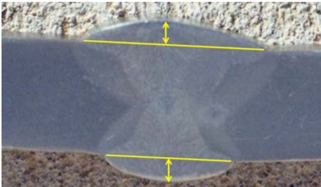
Weld crown or reinforcement is indicated by the double arrows
