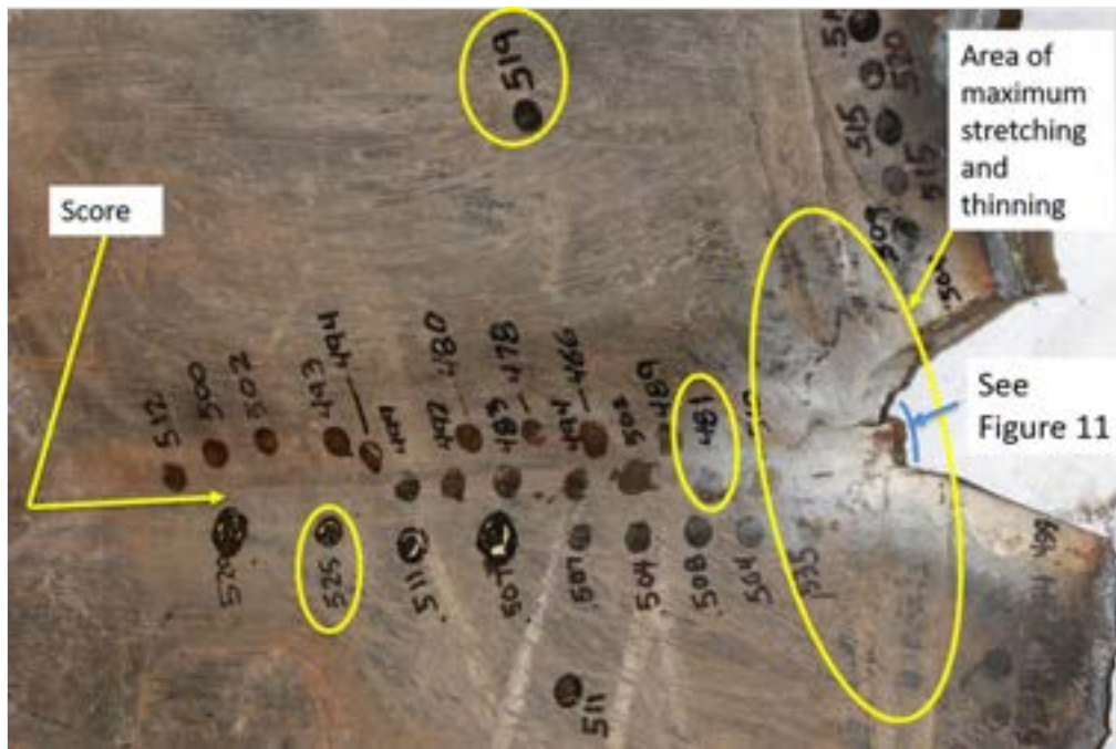
Figure 10 Ultrasonic thickness measurements of the tank shell laboratory coupon that compare the parent metal thickness (0.519-inch to 0.535-inch) to the thickness measured at the depth of the score (0.481-inch to 0.512-inch). 12
