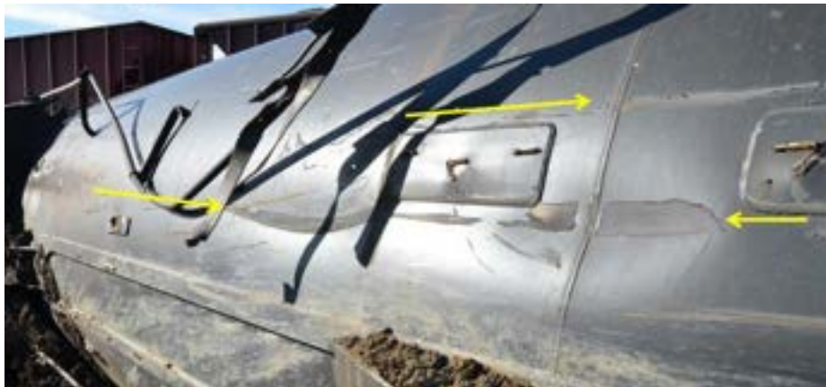
Figure 6 Score – crossing the crown of a circumferential weld. 8
