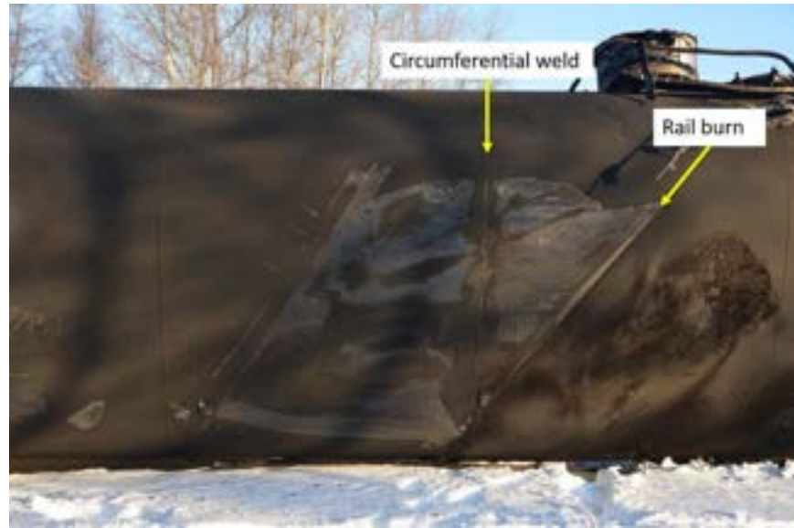
Figure 1 Rail burn – crossing a circumferential weld. 3
