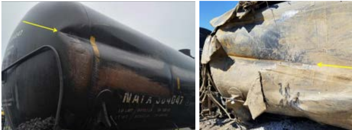
Figure 2 Rail burns and dents crossing circumferential welds. 4
