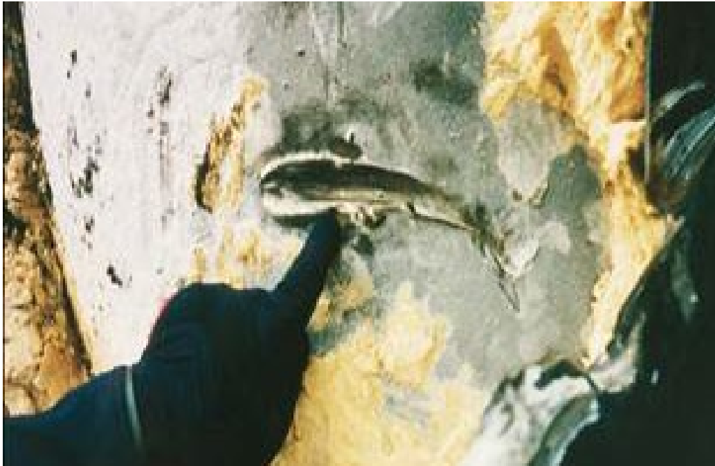
Gouge in head of a chlorine car [Conrail 1995-96].
