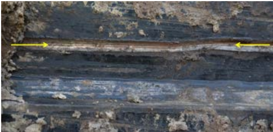
Figure 4 Gouge – indicating removal of metal and a reduction in thickness. 6
