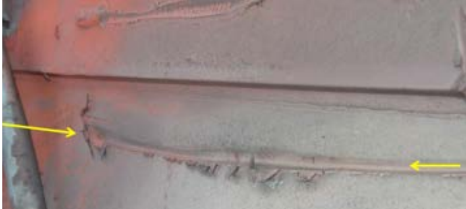
Figure 3 Gouge – indicating removal of metal and a reduction in thickness. 5
