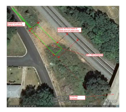
3. Please note that no proposed tower compound should be closer than twenty-five (25) feet from the centerline of tangent main track. Applications will be accepted on a case by case basis up to but no closer than eighteen (18) feet from centerline of tangent main track on Norfolk Southern property.
