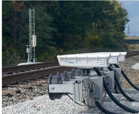
In 2025, we launched our first **Wheel Integrity System**, which builds on our Digital Train Inspection (DTI) technology and leverages synchronized cameras and advanced AI to spot critical wheel defects before they cause problems.
